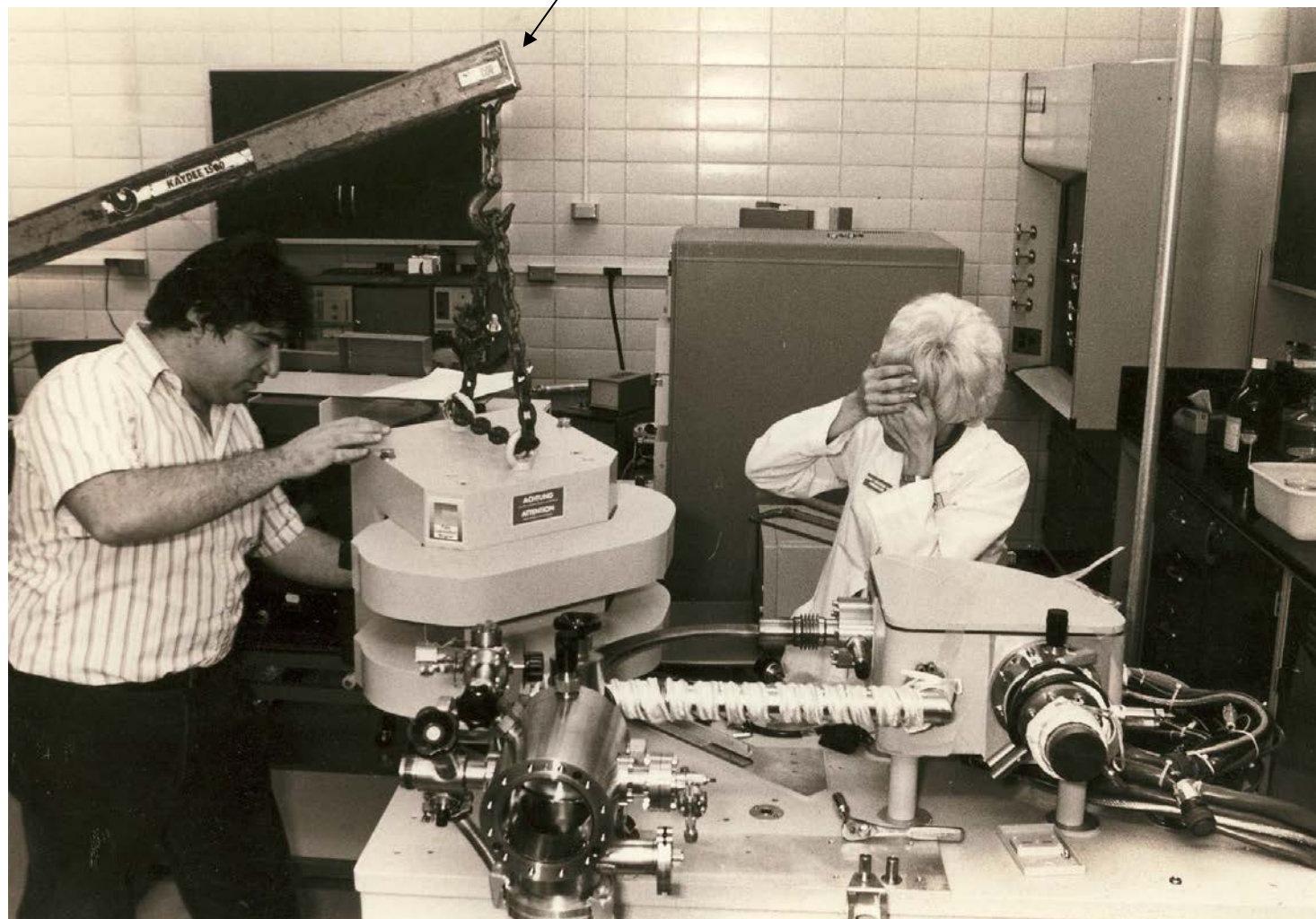
Finnigan-MAT 212 (double focusing magnetic sector mass spectrometer)
