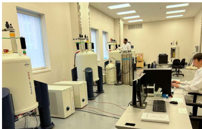
The nuclear magnetic resonance (NMR) laboratory at the National Center for Natural Products Research (NCNPR) at The University of Mississippi School of Pharmacy. The laboratory's construction was partially funded by an ORIP construction grant. Here, natural products chemists use NMR to determine the molecular identity and structure of promising compounds from medicinal plants. Image courtesy of the NCNPR.
