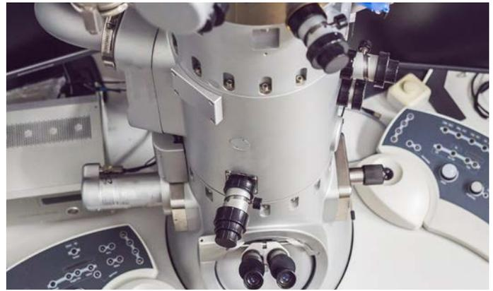
*A transmission electron microscope (TEM). TEMs generate very high-resolution images from thin biological specimens and routinely can magnify objects up to 2 million times. ORIP's S10 program has funded many TEMs, as well as other types of microscopes, since its inception in 1982.*
