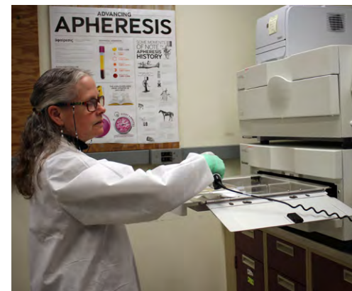
Photo Caption: Instrument used for pathogen reduction and lymphocyte inactivation in blood
